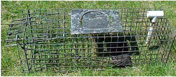
Essentially the bait stick is a half inch PVC pipe. Cut the pipe in six inch lengths and obtain at least one end plug for every cut pipe. Drill holes through the pipe, starting at the ends and working toward the middle until, at least two thirds of the pipe has been drilled. I use a 1/4 inch drill bit. Place the pipe in a vice before drilling. This will make drilling safer by
